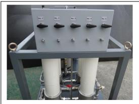
★ Sample line with isolate valve, for purity analyzing at each section.
