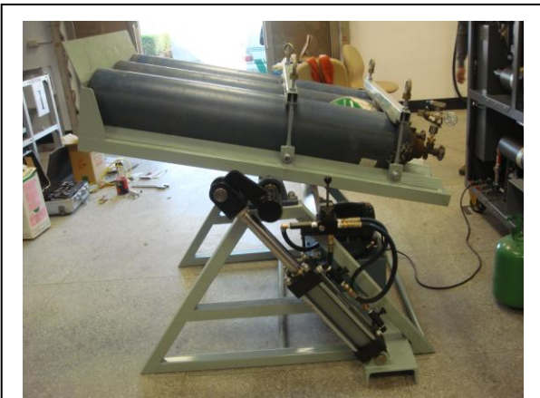
SF 6 Cylinders Moving Angle over 110 degree.
