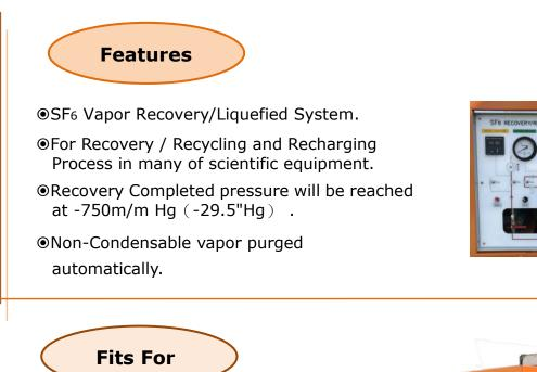
For SF<sub>6</sub> insulating gas in test space.
